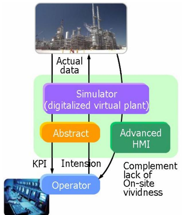
The upper figure shows a typical scheme of a digital plant operation. The plant simulator is placed in the
