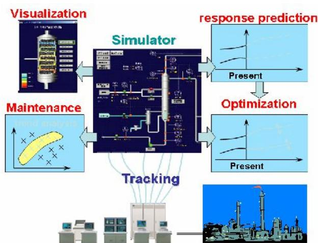
The tracking simulator visualizes the inner status of the plant by interpolating and estimating unmeasured process variables. It also supports plant monitoring and maintenance with calculated KPIs. More importantly, it enables the prediction of the future dynamic behavior of the plant by accelerating calculation in the simulator. Using case simulations with varying parameters, it can help determine the optimal conditions of plant operation in advance.
